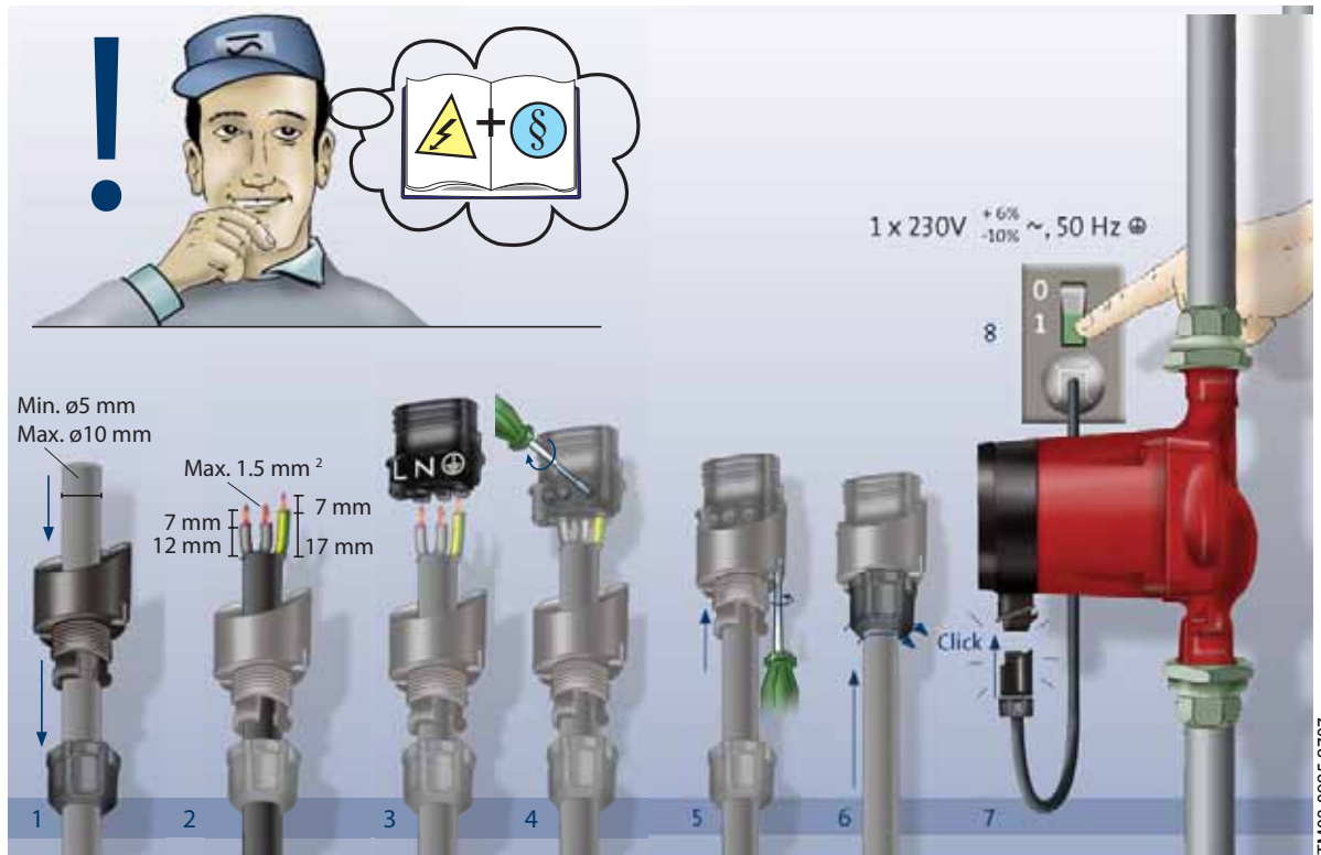
Fig. 6 Electrical connection
