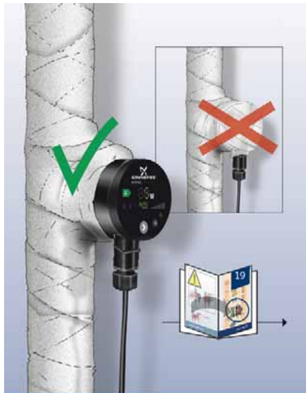
Fig. 5 Insulation of pump housing
